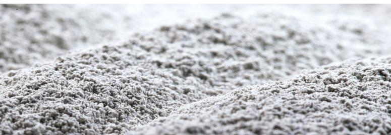
Photoment® is a concrete additive. In a light-dependent photocatalytic reaction at the concrete surface, toxic nitrogen oxides (NO<sub>x</sub>) are rendered harmless. When the application requirements are fulfilled, a superhydrophilic surface is formed and supports the self-cleaning effect of the concrete goods surface.
